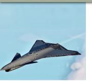
The sleek, tailless, canardequipped design looks to be optimized for high performance while retaining significant lowobservable qualities.
