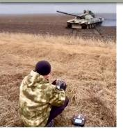
Russia captured converted a Ukrainian tank into remote a controlled vehicle that uses a similar FPV control concept as many kamikaze drones. Such remote controlled tanks could be used in mine-clearing operations, or as a crude 'first-person view' (FPV) tank.
